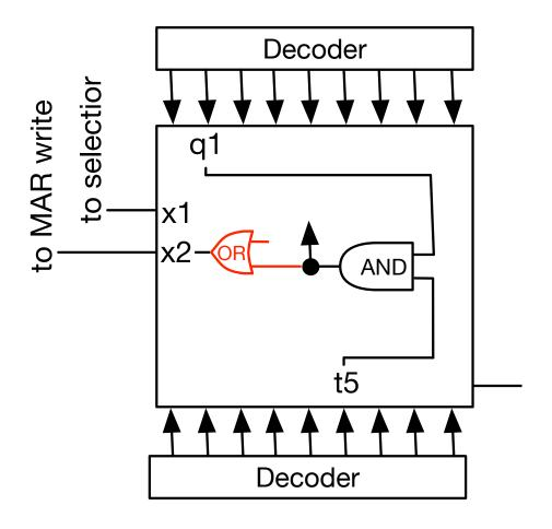
$\label{eq:micro} \begin{array}{ll} \text{Micro instruction:} & q_1 \text{ AND } t_5 \colon \text{ MAR} \leftarrow \text{IR(D)} \\ \\ \text{Set signal to MAR write flag} \end{array}$
