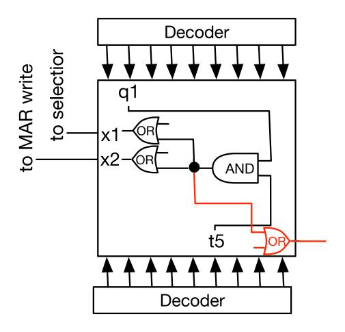
$\label{eq:micro} \begin{array}{lll} \text{Micro instruction:} & q_1 \text{ AND } t_5 \colon \text{ MAR} \leftarrow \text{IR(D)} \\ \\ & \text{Increase micro program time step} \end{array}$
