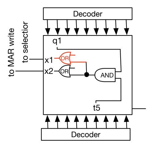
$\label{eq:micro} \begin{array}{ll} \text{Micro instruction:} & q_1 \text{ AND } t_5 \colon \text{ MAR} \leftarrow \text{IR(D)} \\ \\ \text{Set appropriate value to MAR selector} \end{array}$
