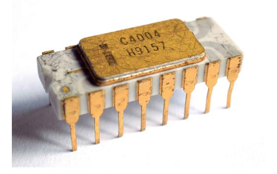
• 4-bit central processing unit, 12 bit address space (4KB)
