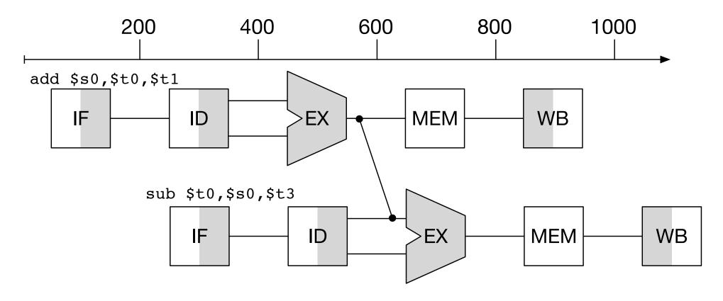
• Add wiring to circuit to directly connect output of ALU for next instruction
