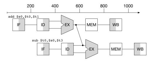
Add wiring to circuit to directly connect output of ALU for next instruction
