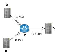
Problem: outgoing link  $C \rightarrow D$  cannot handle aggregate data rate of incoming data from  $A \rightarrow C$  and  $B \rightarrow C$
