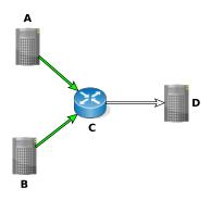
Scenario: A and B both try to send a packet to D at the same time
