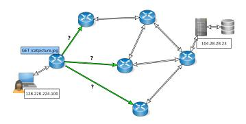
Router has a choice of outgoing links on which to send the packet
