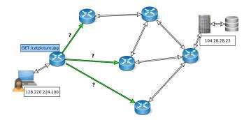
Router has a choice of outgoing links on which to send the packet
