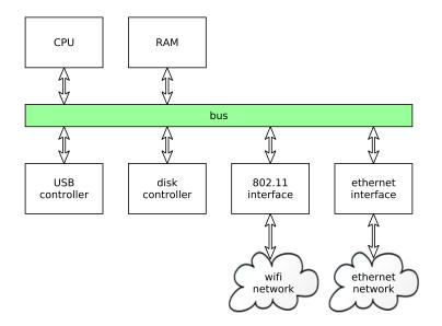
In addition to network interface hardware, a *protocol stack* is needed to allow network applications to communicate over the attached network interface(s)
