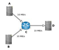
Problem: outgoing link C→D cannot handle aggregate data rate of incoming data from A→C and B→C
